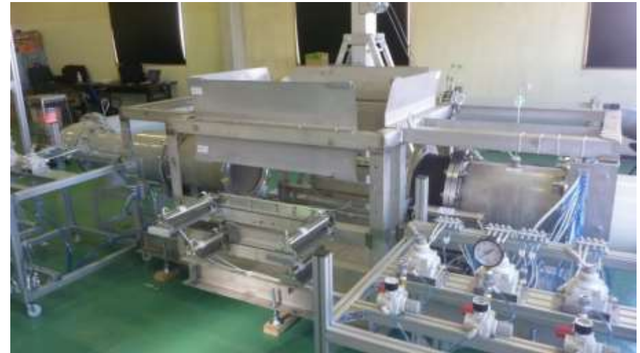
Remote filter replacement equipment
